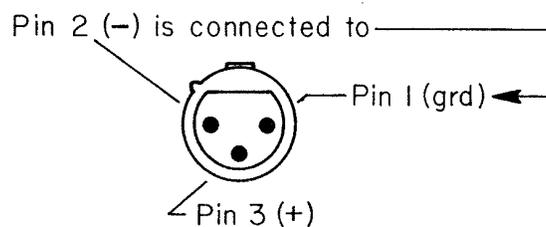
NOTE: Failure to connect Pins 1 and 2 will result in an approximate 50% reduction in gain.
