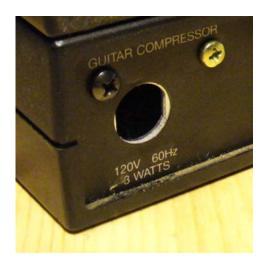
□ Then you can unscrew the barrel plug nut, and remove it from its mounting hole.
